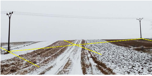
Fig. 5. Decomposition of measuring points between high voltage poles 1 and 2 for the height of 0.3 m.
