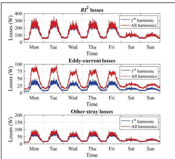
Figure 3.  $RI^2$ , eddy-current and total stray losses with and without considering real measured harmonics for one week
