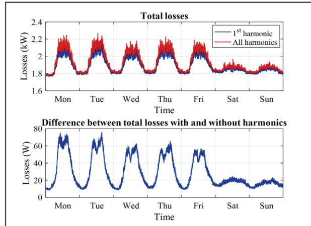
Figure 4. Total losses with and without considering real measured harmonics for one week
