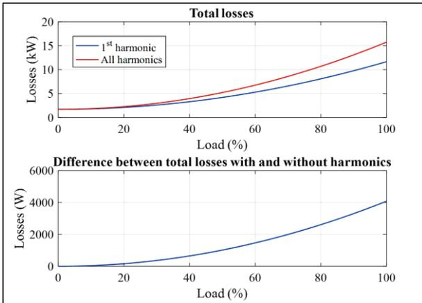
Figure 2. Total losses with and without considering harmonics depending on transformer load
