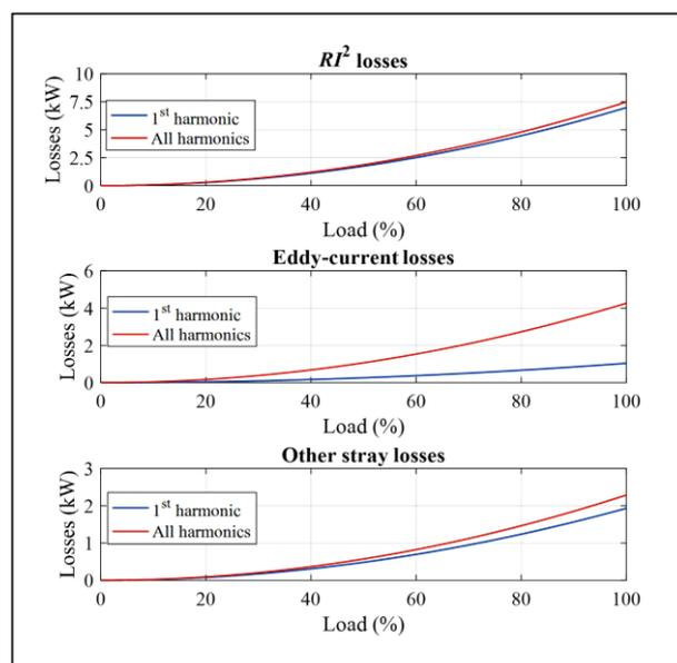
Figure 1.  $RI^2$ , eddy-current and total stray losses with and without considering harmonics depending on transformer load
